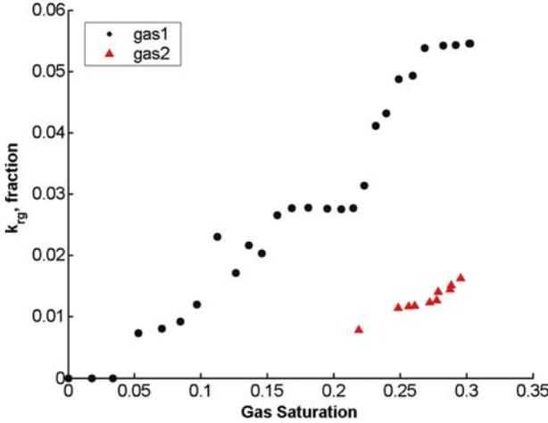
Figure 20. Predicted gas relative permeabilities for a strongly oil-wet system for the saturation path shown in Figure 18.
