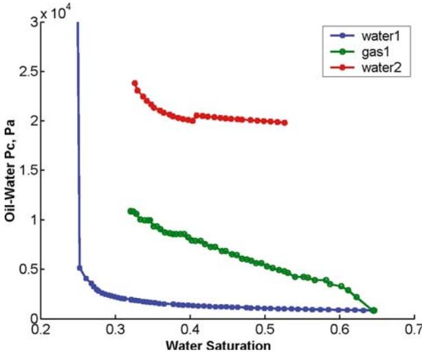
Figure 10. Oil–water capillary pressure for the first water, first gas, and second water injection cycles for the saturation path shown in Figure 5.
