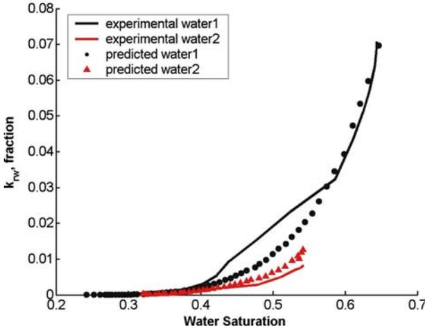
Figure 7. Comparison of measured and predicted water relative permeabilities for the saturation path shown in Figure 5.
