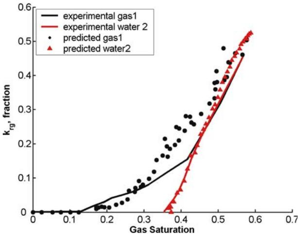
Figure 6. Comparison of measured and predicted gas relative permeabilities for the saturation path shown in Figure 5.
