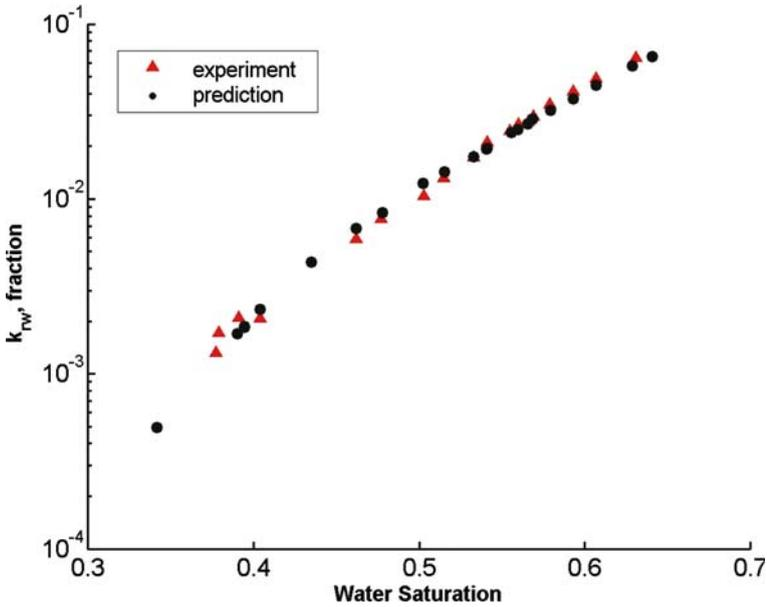
Figure 2. Comparison of measured and predicted water relative permeabilities for the saturation path shown in Figure 1.
