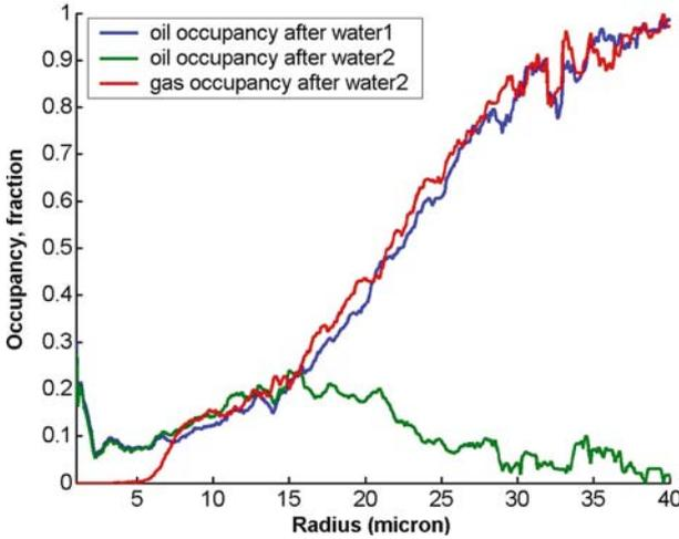
Figure 9. Pore occupancies for the first and second water injection cycles for the saturation path shown in Figure 5.
