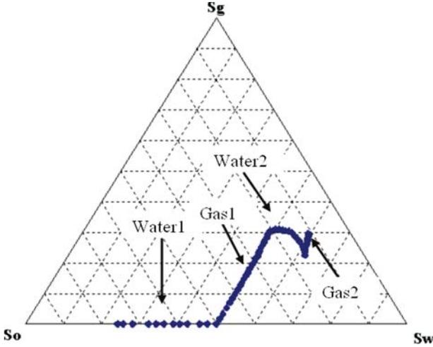
Figure 18. WAG saturation path for a strongly oil-wet system.
