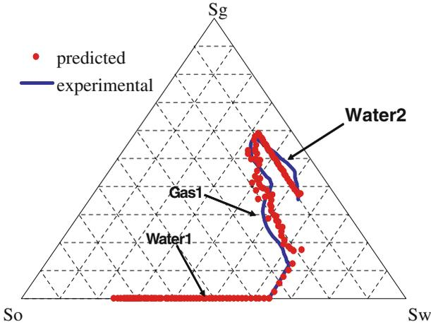
Figure 5. Comparison of measured and tracked saturation paths for cyclic gas and water injection. Experiment 4 – Sample 6 of Oak experiments (Oak, 1990).
