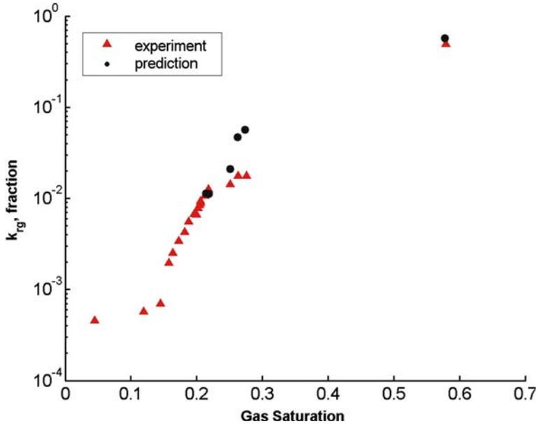
Figure 4. Comparison of measured and predicted gas relative permeabilities for the saturation path shown in Figure 1.
