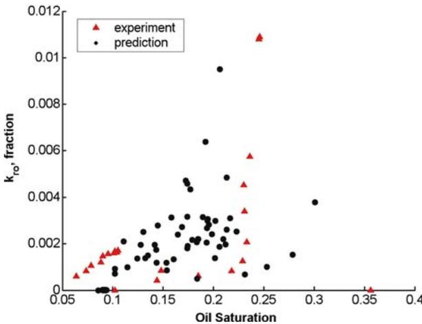
Figure 8. Comparison of measured and predicted oil relative permeabilities for gas 1 and water 2 cycles shown in Figure 5.
