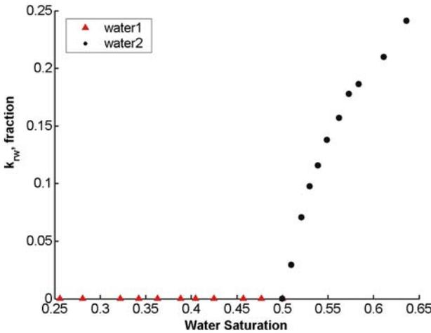
Figure 21. Predicted water relative permeabilities for a strongly oil-wet system for the saturation path shown in Figure 18.
