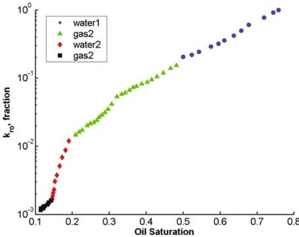
Figure 19. Predicted oil relative permeability for a strongly oil-wet system for the saturation path shown in Figure 18.
