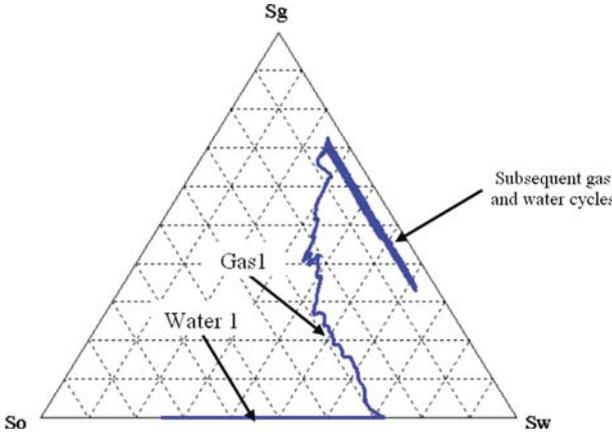
Figure 16. WAG saturation path for a water-wet system.
