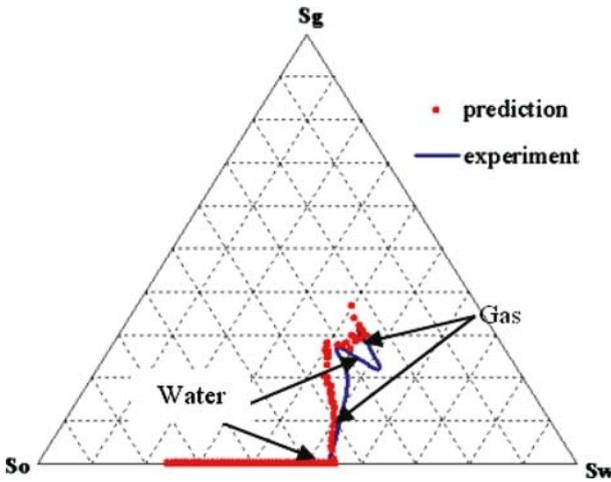
Figure 14. Comparison of measured (Element *et al.*, 2003) and tracked saturation paths.
