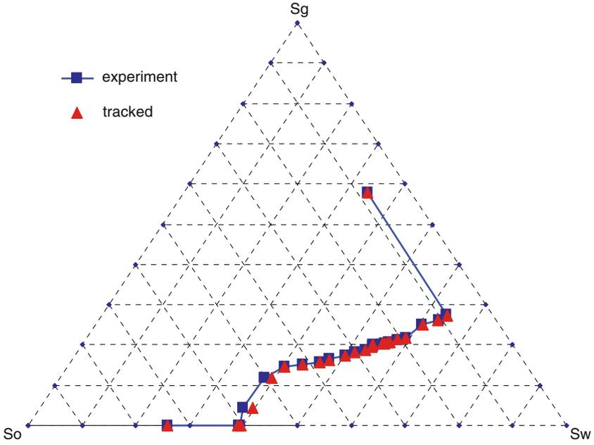
Figure 1. Comparison of measured and tracked saturation paths for simultaneous water and gas injection. Experiment 14 – Sample 13 of Oak experiments (Oak, 1990).
