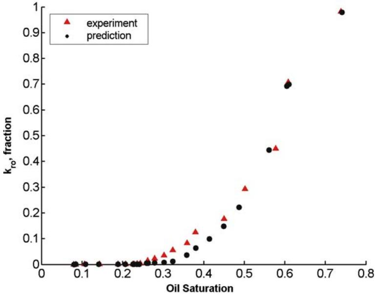
Figure 3. Comparison of measured and predicted oil relative permeabilities for the saturation path shown in Figure 1.
