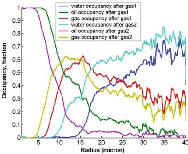
Figure 22. Pore occupancies for first and second gas injection cycles in a strongly oil-wet medium for the saturation path shown in Figure 18.
