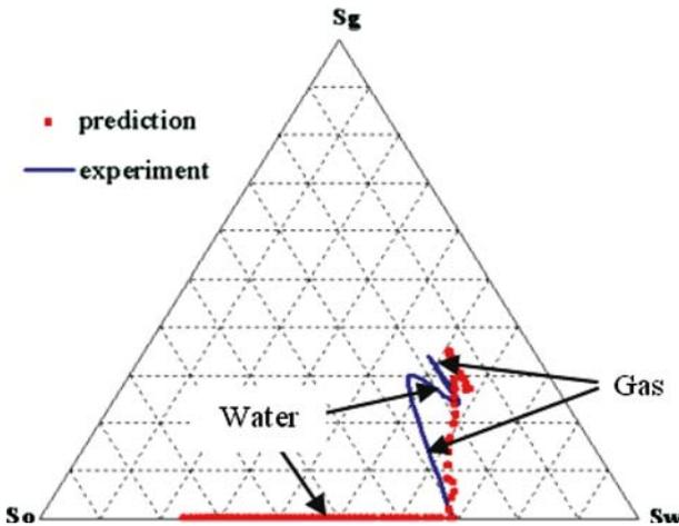
Figure 11. Comparison of measured (Egermann *et al.*, 2000) and tracked saturation paths.
