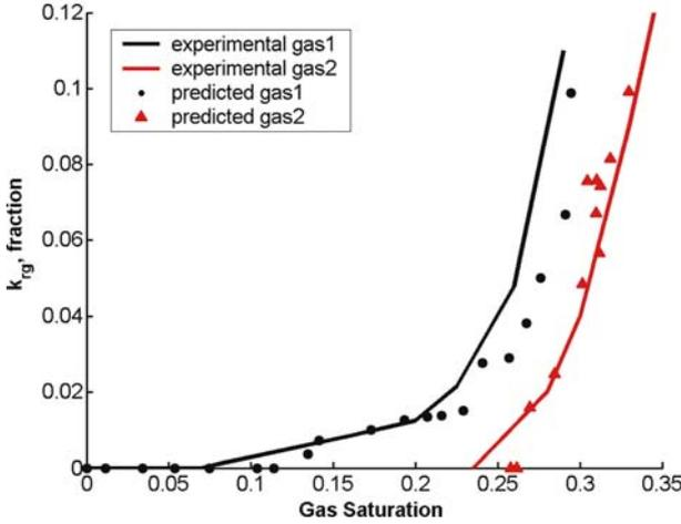
Figure 12. Comparison of measured (Egermann *et al.*, 2000) and predicted gas relative permeabilities for the saturation path shown in Figure 11.
