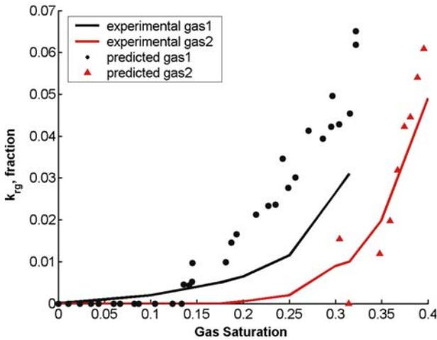
Figure 15. Comparison of measured (Element *et al.*, 2003) and predicted gas relative permeabilities for the saturation path shown in Figure 14.
