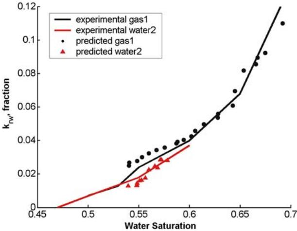
Figure 13. Comparison of measured (Egermann *et al.*, 2000) and predicted water relative permeabilities for the saturation path shown in Figure 11.
