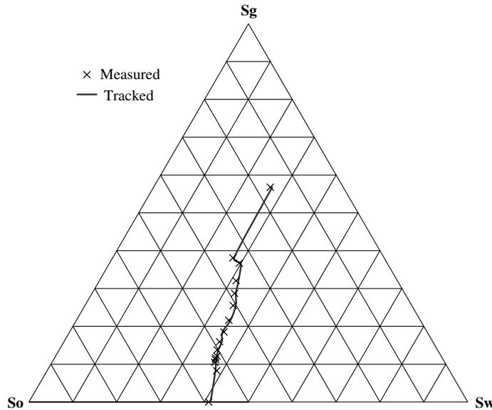
Figure 11. Saturation path for a steady-state experiment by Oak (1990) for gas injection into oil and water (crosses). The network model undergoes a series of displacements of water or oil by gas to reproduce a similar path (line).
