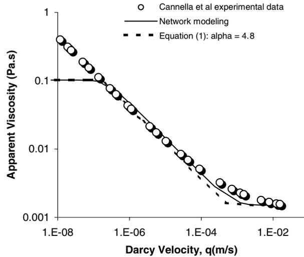
Figure 4. Comparison between network simulations (lines) and Cannella *et al.* (1988) experiments on Berea sandstone (circles). The dashed line is an empirical fit to the data, Equation (1), using an adjustable scaling factor.
