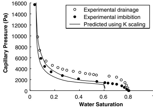
Figure 6. Comparison between predicted capillary pressures and experimental data by Dury *et al.* (1998). The size of the elements in the Berea network is modified using a scaling factor based on absolute permeability and the predictions are poor, indicating that the pore size distribution needs to be adjusted to match the data.
