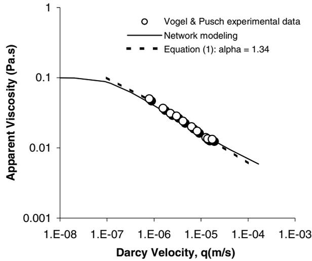
Figure 2. Comparison between network simulations (line) and the Vogel and Pusch (1981) experiments on a sand pack (circles). The dashed line is an empirical fit to the data, Equation (1), using an adjustable scaling factor  $\alpha$ .
