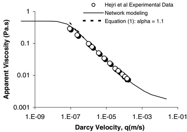
Figure 3. Comparison between network simulations (line) and the Hejri *et al.* (1988) experiments on a sand pack (circles). The dashed line is an empirical fit to the data, Equation (1), using an adjustable scaling factor  $\alpha$ .
