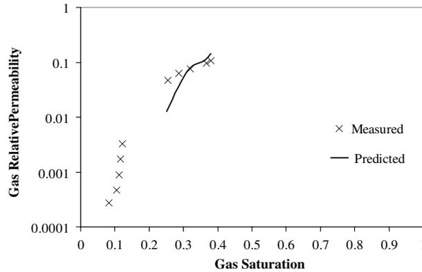
Figure 13. Experimentally measured gas relative permeability for gas injection after waterflooding (crosses) from Oak (1990) compared to network model predictions (line).
