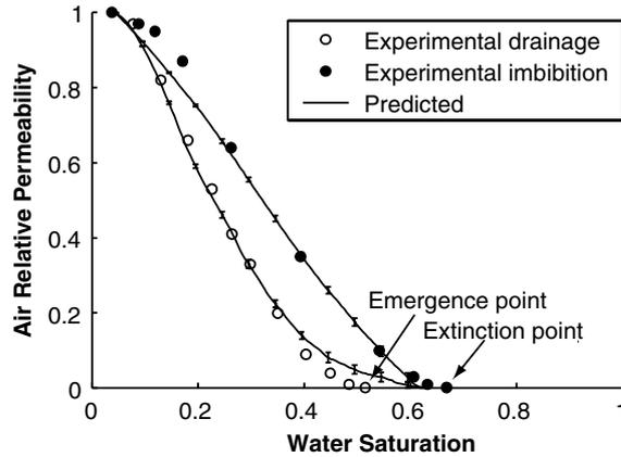
Figure 8. Comparison of network model air relative permeability predictions to experimental data measured on a sand pack by Dury *et al.* (1998). The flooding cycles shown are secondary drainage and tertiary imbibition (main cycles) and the experimental data are obtained using the stationary liquid method. The emergence point represents when gas first starts to flow during gas invasion (drainage) and the extinction point is where gas ceases to flow during imbibition.
