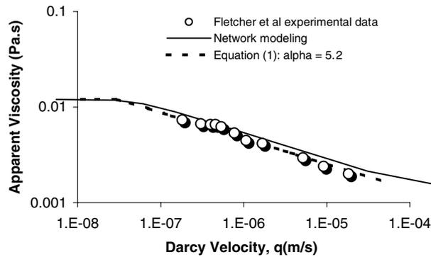
Figure 5. Comparison between network simulations (line) and the experiments of Fletcher *et al.* (1991) on Berea sandstone (circles). The dashed line is an empirical fit to the data, Equation (1), using an adjustable scaling factor  $\alpha$ .
