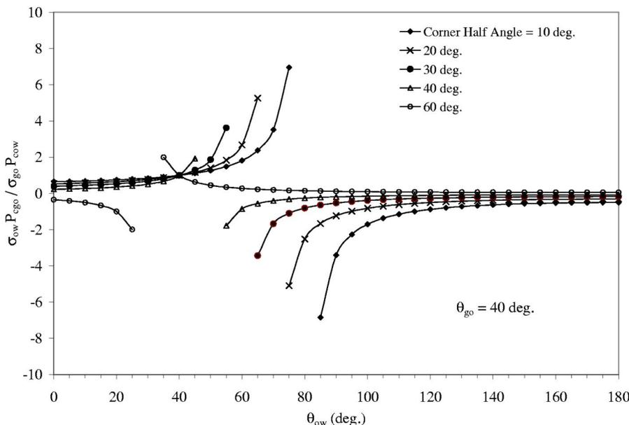
FIG. 10. Effects of corner half angle and oil/water contact angle on oil layer stability for  $\theta_{go}=40$  deg.
