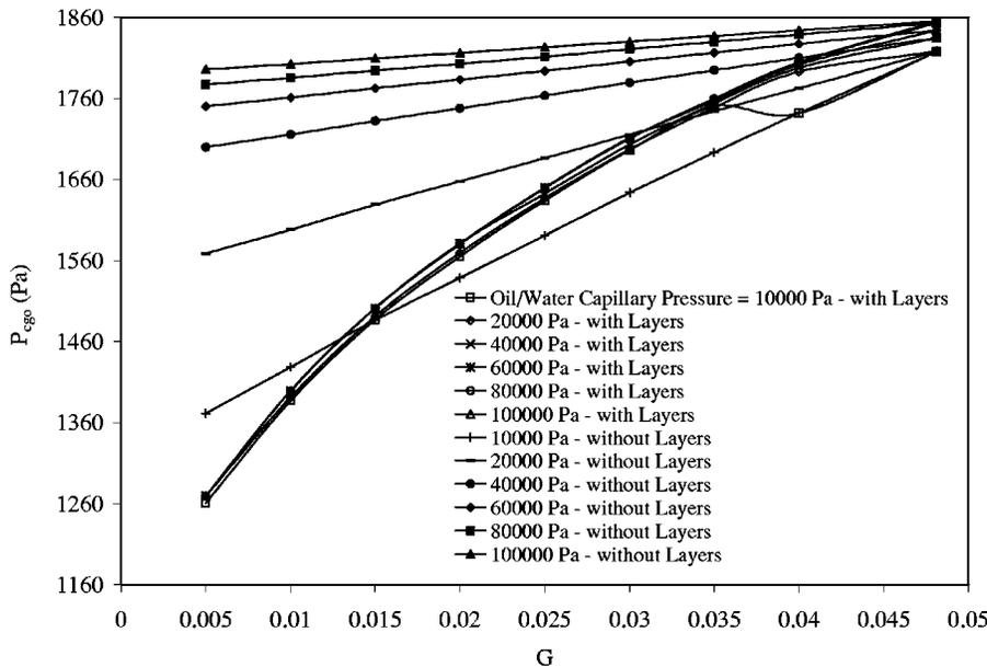
FIG. 7. Threshold gas/oil capillary pressures for system *D*.
