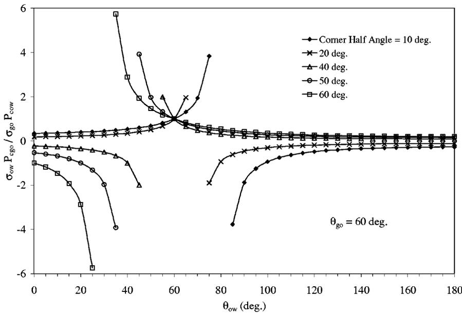
FIG. 11. Effects of corner half angle and oil/water contact angle on oil layer stability for  $\theta_{go} = 60$  deg.
