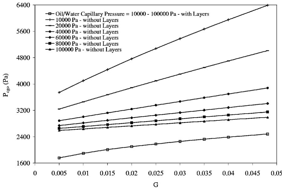
FIG. 5. Threshold gas/oil capillary pressures for system B.
