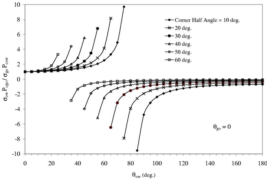
FIG. 9. Effects of corner half angle and oil/water contact angle on oil layer stability for  $\theta_{go}=0$ .
