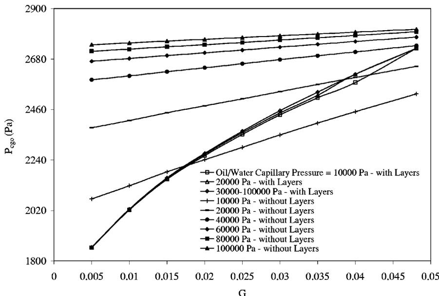
FIG. 6. Threshold gas/oil capillary pressures for system C.
