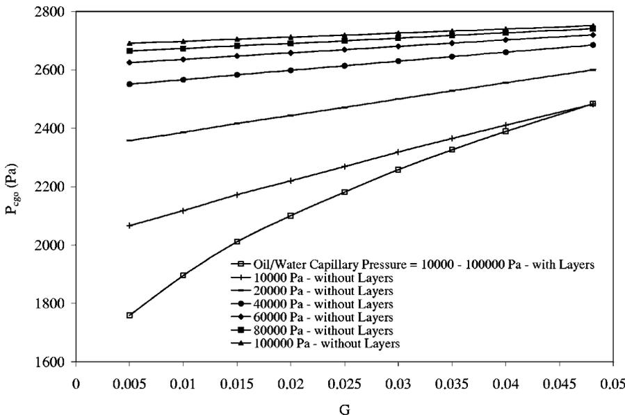
FIG. 4. Threshold gas/oil capillary pressures for system A.
