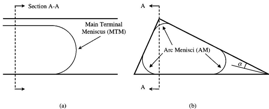
FIG. 1. Different types of interface (a) main terminal meniscus (MTM), and (b) arc menisci (AMs) in the corners of a capillary element of triangular cross section.  $\alpha$  is the corner half angle [5].
